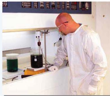
Performing the etch and die removal process
